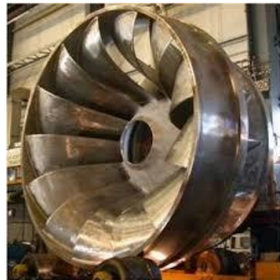
Turbine hydraulique (Francis)
